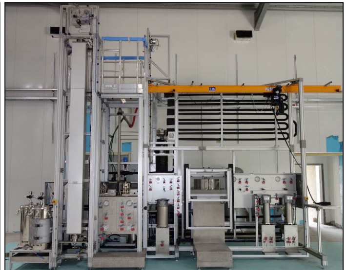
Supercritical fluid extraction lab system for APEX company in Tunisia, optimized for Supercritical CO 2 and capacity to work with other type of green solvents.
