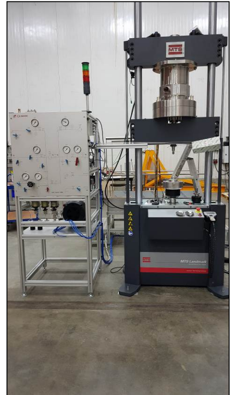
Traction machine for GRT GAZ customer in France, allowing traction/compression tests on specimens under pressure and temperature
